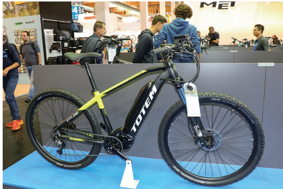
▲ Totem Czech plant's e-MTBs feature Panasonic drive systems and SR Suntour suspension forks.
