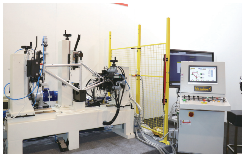
▲ The first piece of equipment that Bike Machinery / Mair has authorized Jui Chih to produce: the Proxima fully automatic bicycle frame alignment machine.
