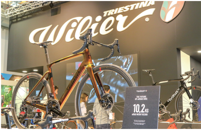
▲ Wilier's Cento 10 Hybrid features fully hidden cables, weighs a mere 10.2kg, is equipped with Mahle's rear wheel drive motor system, and has a retail price of €11,200.
