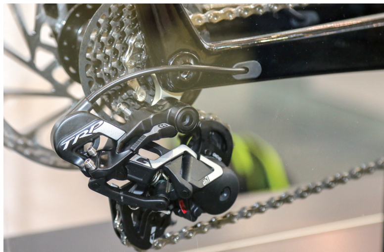
▲ Derailleurs and shifters for downhill bikes developed jointly by TRP and its sponsored cyclist Aaron Gwin. The components' hall lock and ratchet clutch have a special design intended to meet the requirements of downhill bikes.
